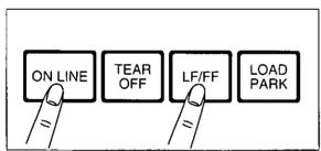
press [LF/FF] once to advance the paper one micro line (1/216"). Holding the switches will advance the paper continuously until you release the switches. Using the Micro Line Feed within 5" from the top of your paper automatically stores the position as the Top of Form.
