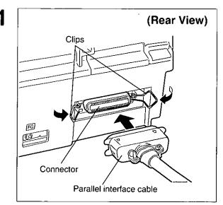
Attach the other end of the parallel interface cable from your computer to your printer and secure the printer clips.
