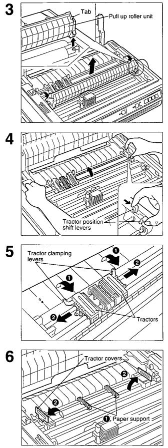
Remove the pull up roller unit by grabbing the tabs at both ends and gently rotating forward until you feel it release, then lift up.
