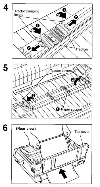
• Unlock the tractors by pulling the tractor clamping levers forward.
