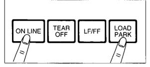
With paper installed, while pressing **ON LINE**, press **LOAD/PARK**) once to reverse the paper one micro line (1/216"). Holding the switches will reverse the paper continuously until you release the switches. Using the Reverse Micro Line Feed within 5" from the top of your paper automatically stores the position as the Top of Form.
