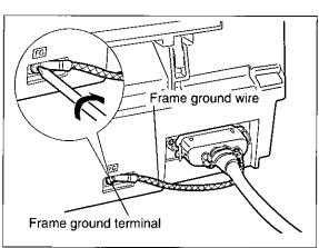
If the cable has a frame ground wire, connect it to the frame ground terminal.
